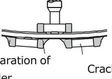
Separation of solder<br>Crack |
