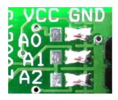
The I2C-TMP features three address pins to allow up to 27 devices to be addressed on a single bus interface.
