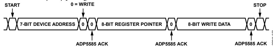
Figure 23. I 2 C Single Byte Write Sequence
