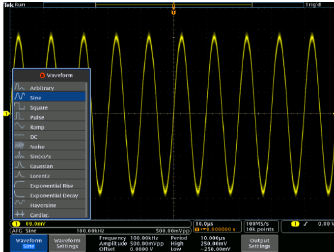
Waveform type selection in the integrated AFG.
