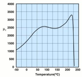
Measured on an 18/10/6mm toroid at 100kHz.
