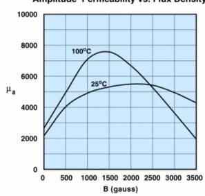
Measured on an 18/10/6mm toroid at 10kHz.
