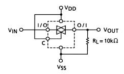
$$R_{ON} = 10 \times \frac{(V_{IN} - V_{OUT})}{V_{OUT}} (k\Omega)$$
