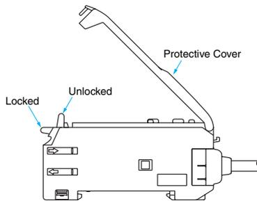
**Note:** To maintain the fiber properties, confirm that the lock is released before removing the fiber.
