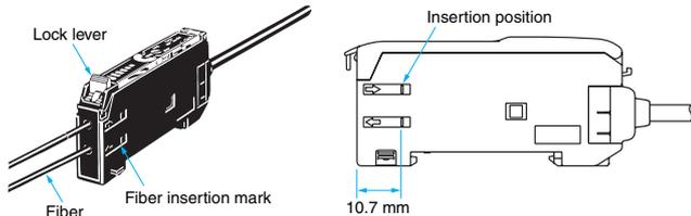
**Note:** If one of the fibers from the Fiber Unit has a white line, such as with a Coaxial Sensor, that fiber is for the Emitter. Insert it into the Emitter section. Refer to Dimensions for the Fiber Unit to see if there is an Emitter fiber.
