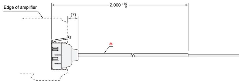
\* E3X-CN12: **2.6 dia. cable / 1 conductor** / Standard length: 2 m (Conductor cross section: 0.2 mm<sup>2</sup> (AWG24), Insulator diameter: 1.1 mm)
