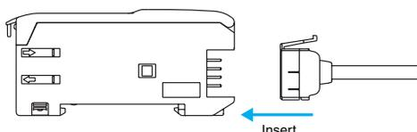
2. Join Amplifier Units together as required after all the Master and Slave Connectors have been inserted.
