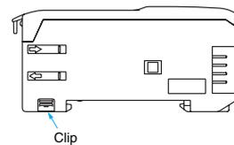
The clip can also be removed using the following mechanism, which is incorporated in the construction of the section underneath the clip.
