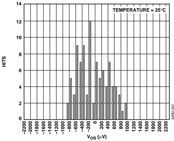
Figure 19. Vos Distribution, MSOP, Temperature = 25°C
