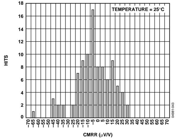
Figure 15. CMRR Distribution, -8 V to +28 V Common Mode
