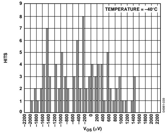
Figure 21. Vos Distribution, MSOP, Temperature = -40°C
