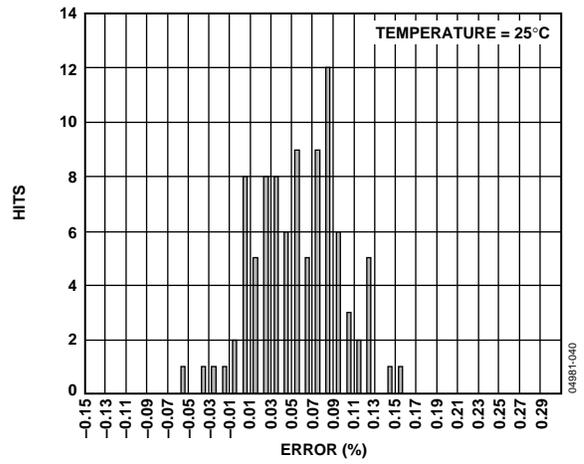
Figure 22. MSOP Gain Accuracy, Temperature = 25°C
