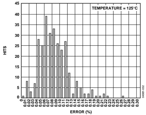
Figure 35. Gain Accuracy, SOIC, Temperature = 125°C
