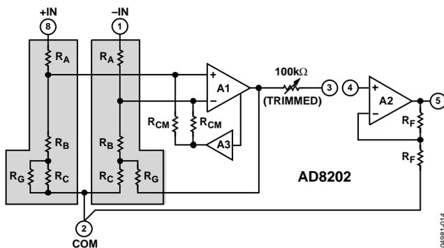
Figure 40. Simplified Schematic
