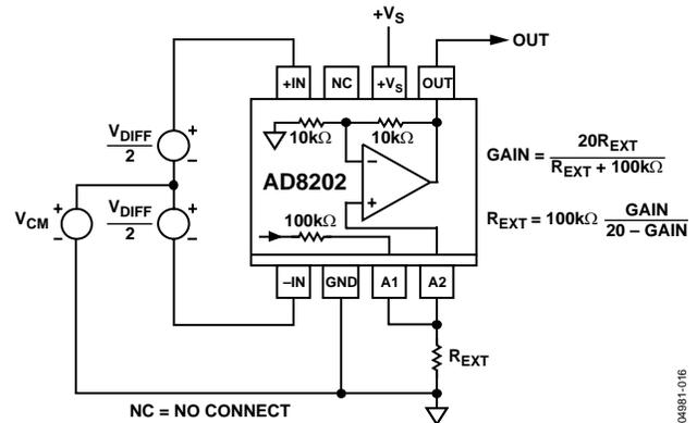
Figure 43. Adjusting for Gains Less than 20
