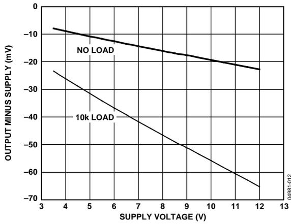
Figure 12. Output Minus Supply vs. Supply Voltage
