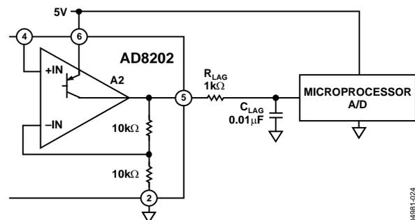
Figure 51. Recommended Circuit for Driving CMOS A/D
