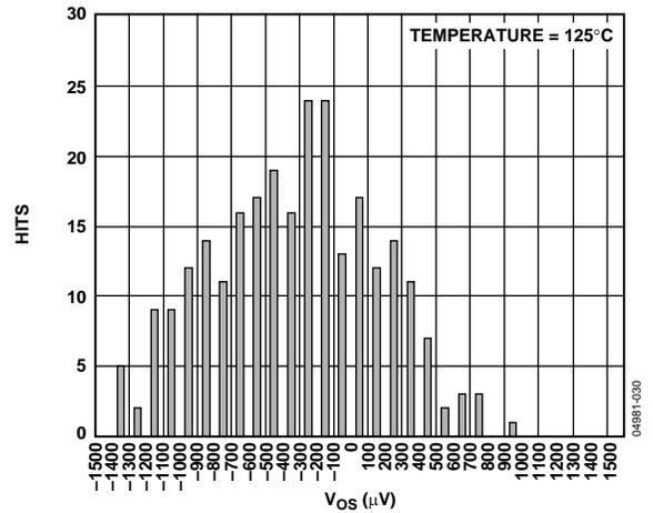
Figure 29. Vos Distribution, SOIC, Temperature = 125°C
