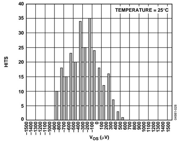
Figure 28. Vos Distribution, SOIC, Temperature = 25°C
