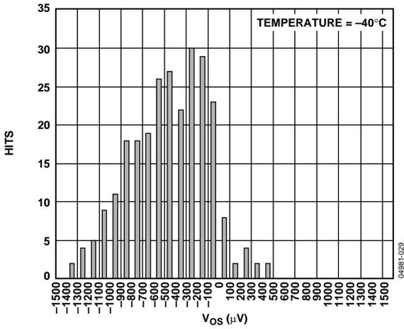
Figure 30.  $V_{OS}$  Distribution, SOIC, Temperature = -40°C
