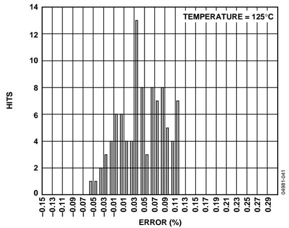
Figure 23. MSOP Gain Accuracy, Temperature = 125°C
