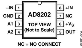
Figure 4. Pin Configuration
