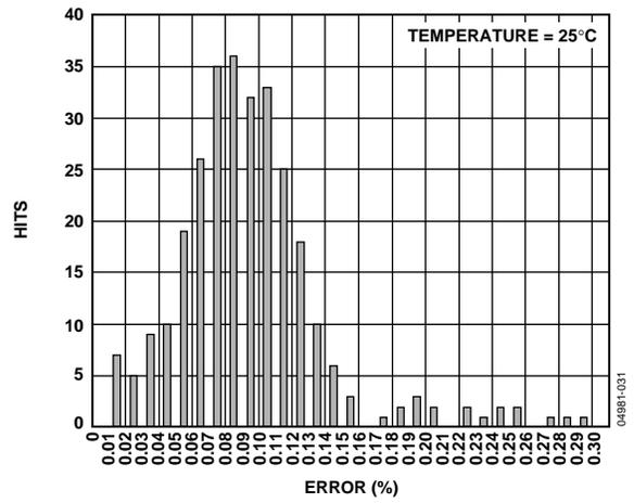
Figure 34. Gain Accuracy, SOIC, Temperature = 25°C
