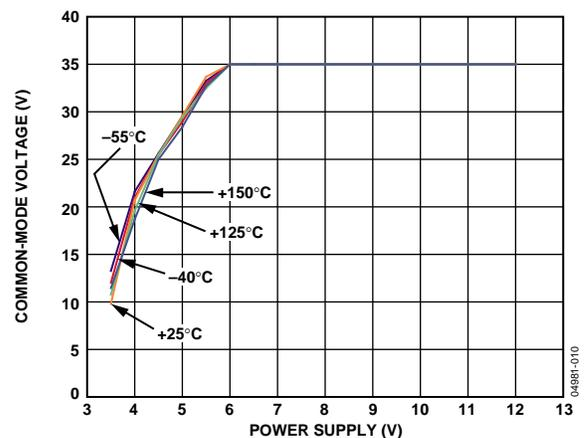
Figure 10. Positive Common-Mode Voltage vs. Voltage Supply
