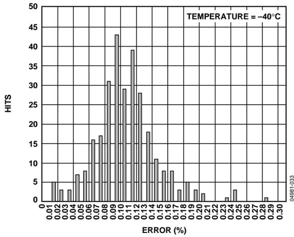
Figure 36. Gain Accuracy, SOIC, Temperature = -40°C
