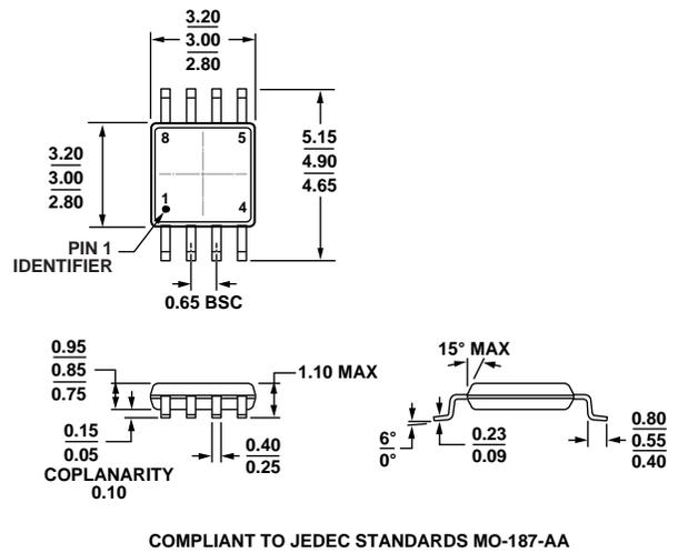
Figure 53. 8-Lead Mini Small Outline Package [MSOP] (RM-8)
