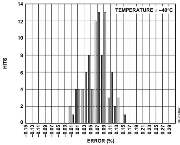
Figure 24. MSOP Gain Accuracy, Temperature = -40°C
