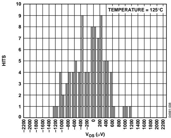
Figure 20. Vos Distribution, MSOP, Temperature = 125°C
