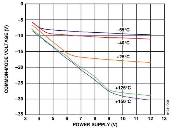
Figure 9. Negative Common-Mode Voltage vs. Voltage Supply
