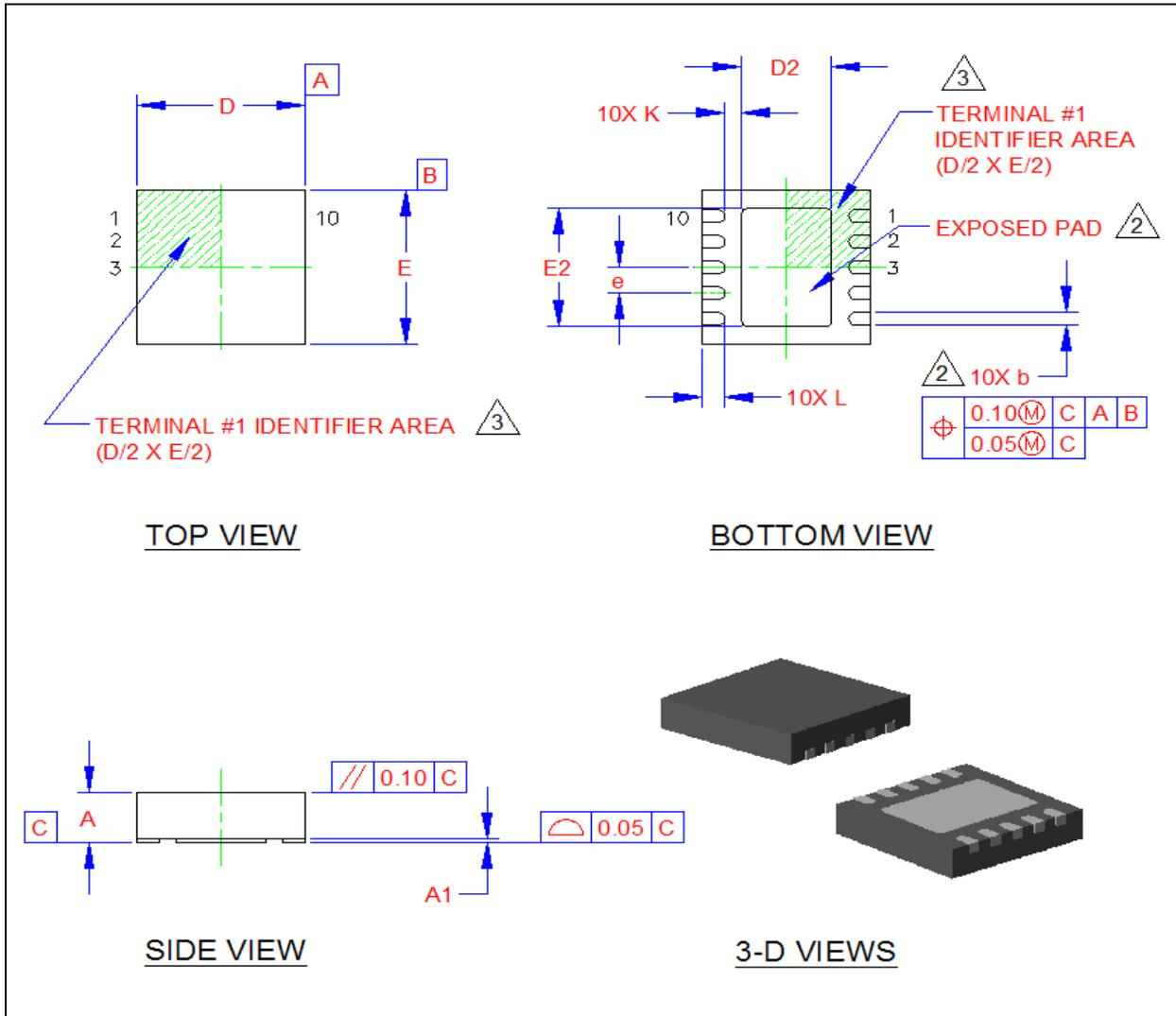
Figure 6.1 10-Pin DFN 3mm x 3mm Package Drawings
