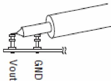
**Figure 2. Proper Input/Output Ripple Measurement Technique**
