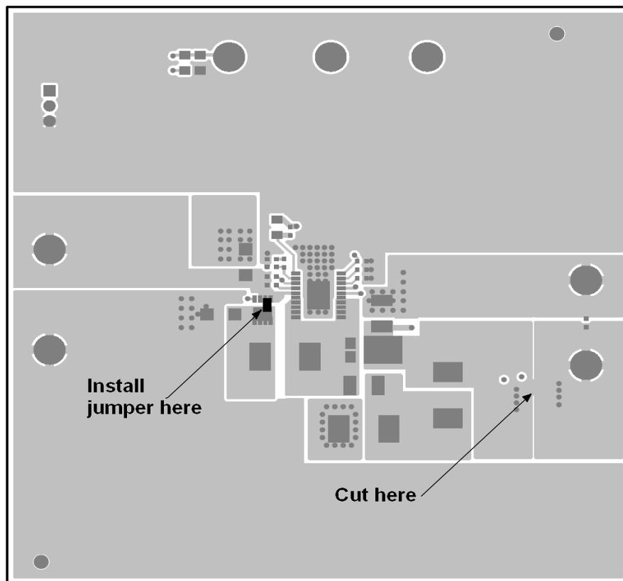
**Figure 3. Instructions for using Disconnect MOSFET at the Output Side**
