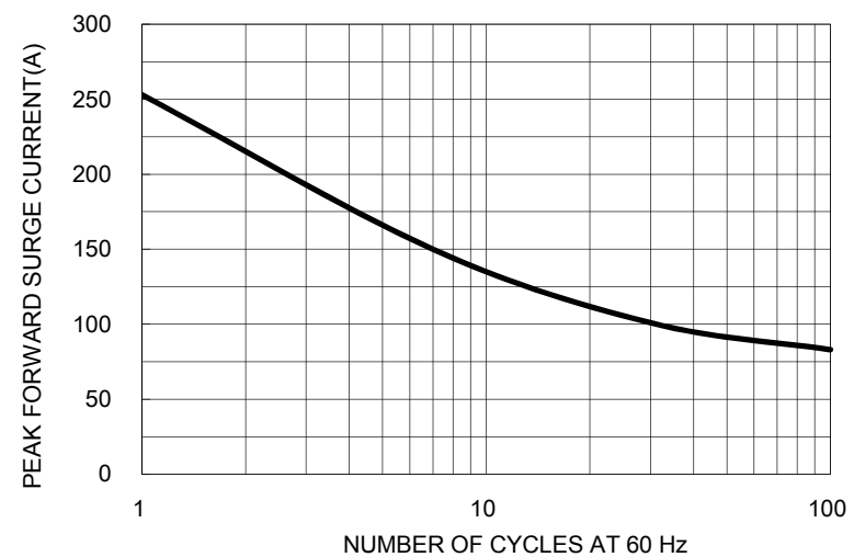
FIG. 3- MAXIMUM NON-REPETITIVE FORWARD SURGE CURRENT
