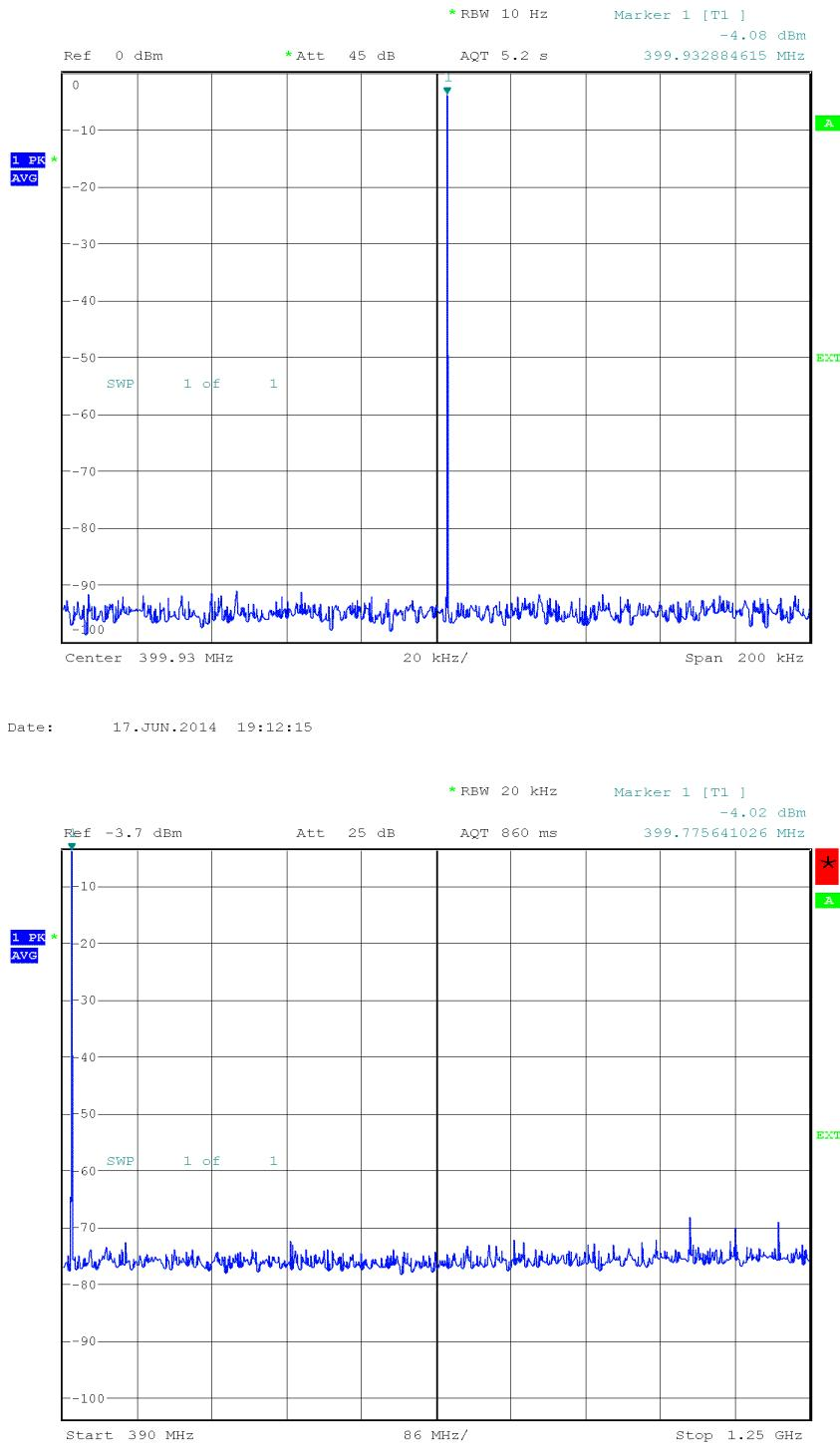
Figure 4. DC2085 Results. Close-In (Top) and Wideband (Bottom)
