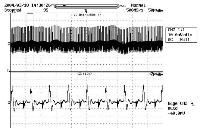
**Figure 24** – Ripple, 75 VDC, Full Load.
