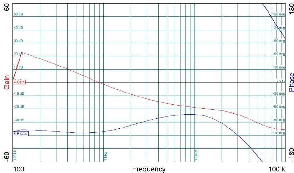
**Figure 27** - Gain-Phase Plot, 36 VDC, Light Load (100 mA).
