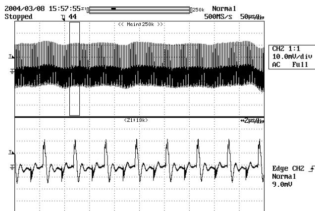
**Figure 23** - Ripple, 57 VDC, Full Load.
