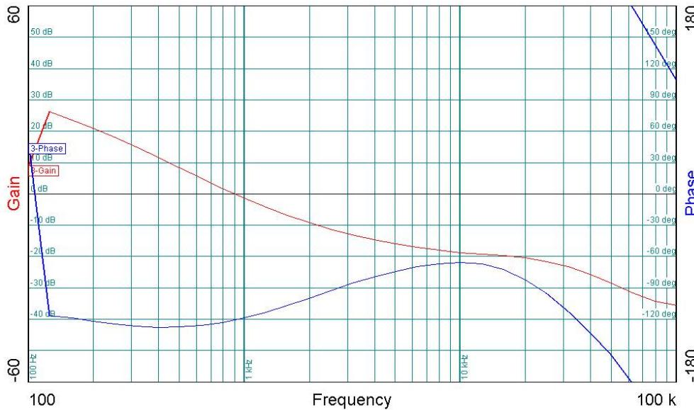
**Figure 29** - Gain-Phase Plot, 57 VDC, Light Load (100 mA).
