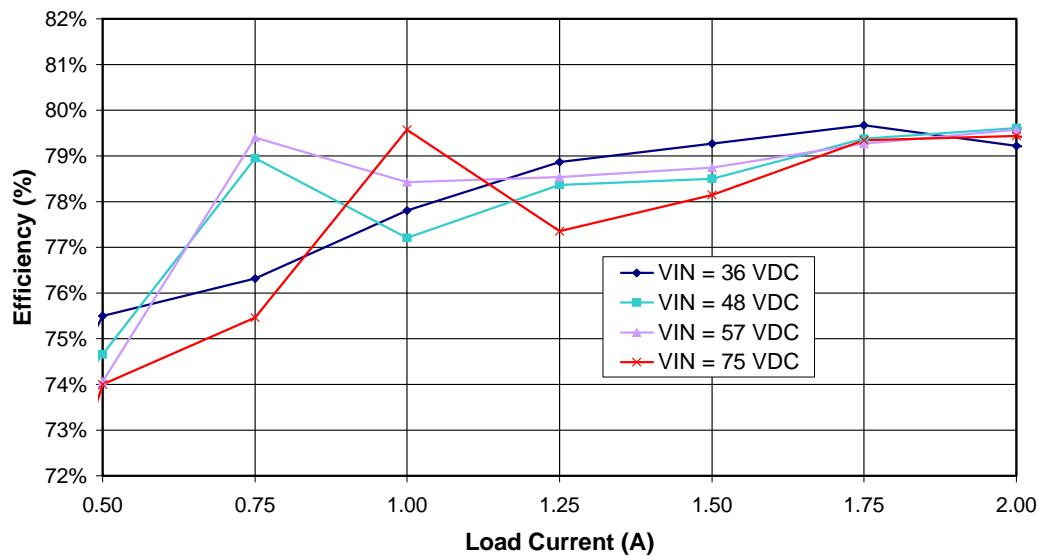
**Figure 7 - Efficiency vs. Output Load, Room Temperature.**
