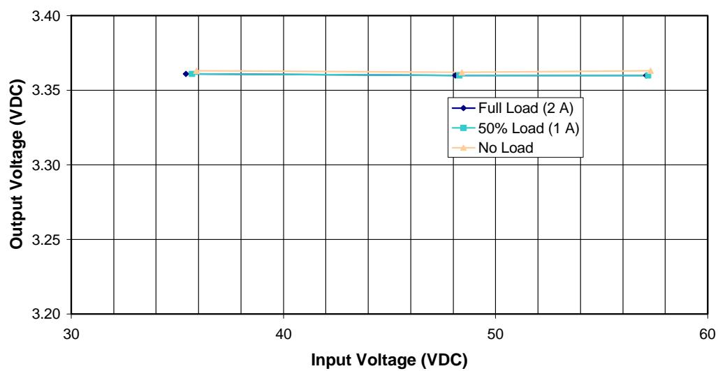
**Figure 9** - Line Regulation, Room Temperature.
