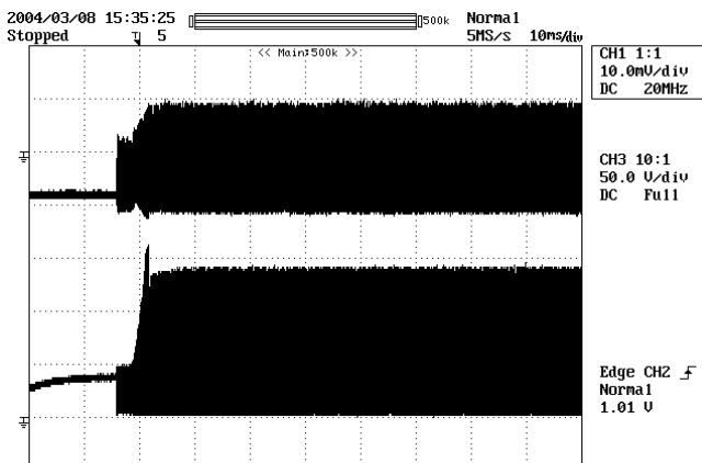
**Figure 15 – 36 VDC Input, 2 A Resistive Load.**
