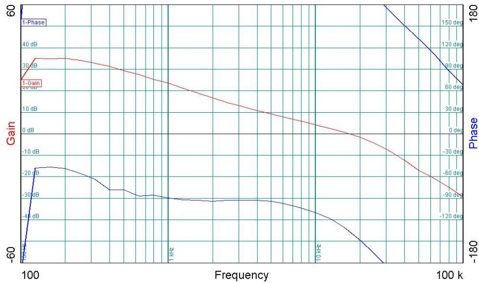
**Figure 28** - Gain-Phase Plot, 57 VDC, Light Load (100 mA).
