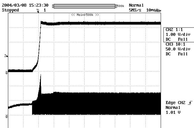
**Figure 13 - Start-up Profile, 36 VDC, No Load (Worst-case).**
