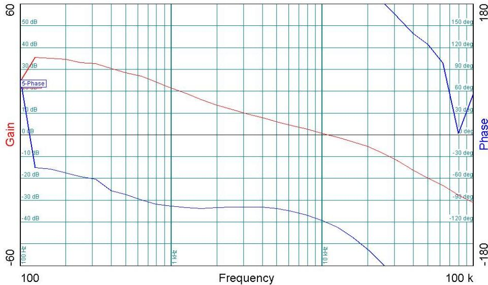
**Figure 26** - Gain-Phase Plot, 36 VDC, Maximum Load (2 A).
