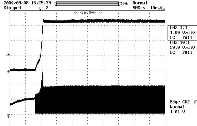
**Figure 14 - Start-up Profile, 57 VDC, No Load (Worst-case).**
