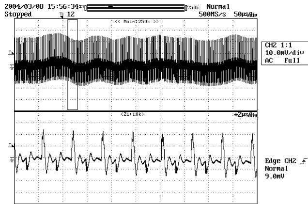
**Figure 21** - Ripple, 36 VDC, Full Load.
