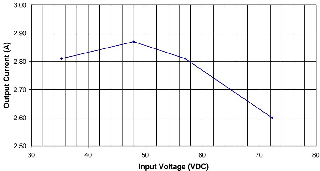
**Figure 10** - Maximum Output Overload Current, Room Temperature.
