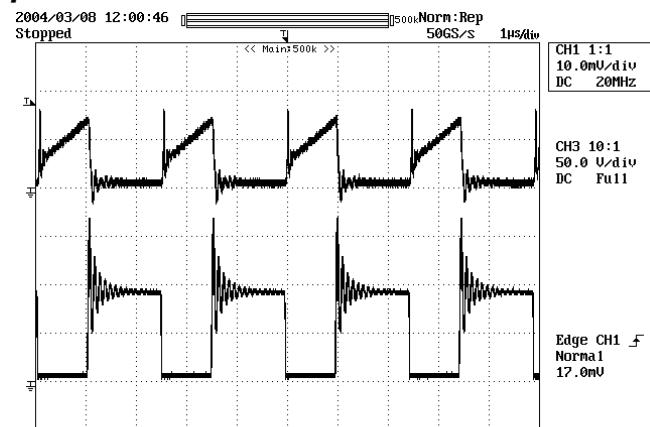
**Figure 12** – 57 VDC, Full Load.
