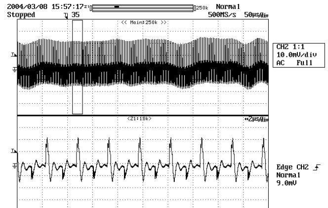
**Figure 22** - Ripple, 48 VDC, Full Load.
