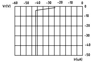
FIG.3a RED REVERSE CURRENT VS. REVERSE VOLTAGE.
