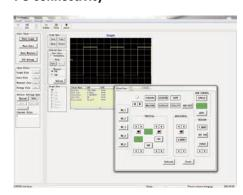
PC software is provided (free download at B&K Precision's website at www.bkprecision.com) for seamless integration between the oscilloscope and PC. Capture and transfer waveforms, screen images, setups and measurement results to a Windows PC via the USB device port on the back of the instrument. A USB host port on the front and rear allows for quick and easy screen saving.
