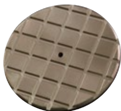
Polishing Puck showing grooves for wet polish
