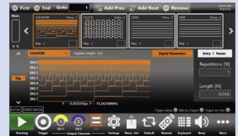
Digital Pattern Generation (DPG functionality)
