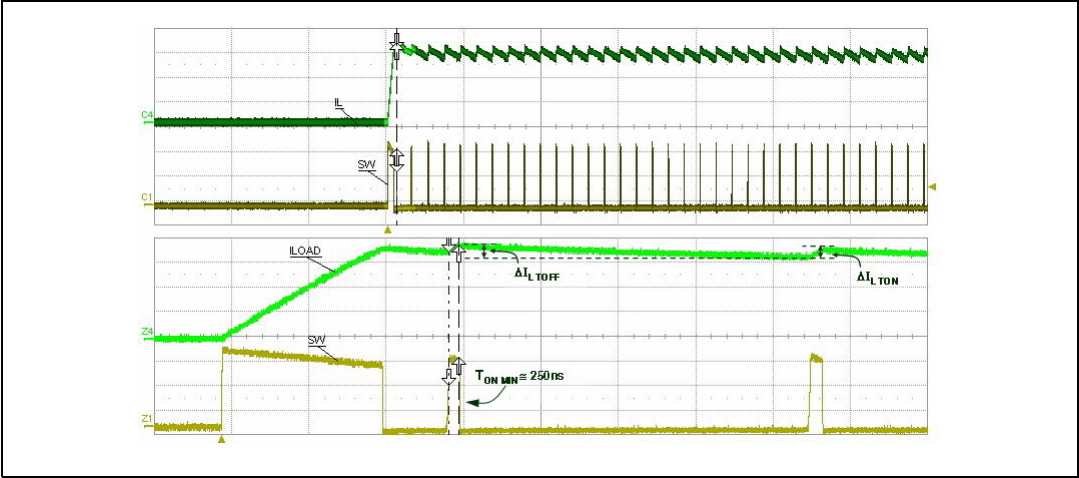
Figure 19. Short-circuit current V_{IN} = 12\text{ V}
