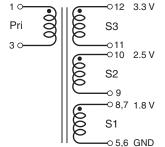
The secondary windings are to be connected in series on the board by connecting pins 9, 8 and 7 together and pins 11 and 10 together. Outputs at pins 12, 11,10 and 8,7 are referenced to ground (pins 5,6).
