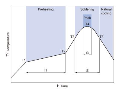
Preheating Soldering Peak Temp. Temp. Time Time Temp. Time T2 Т3 **T4** t3 150°C 180°C 60 to 120s 230°C 30s 260°C 10s
