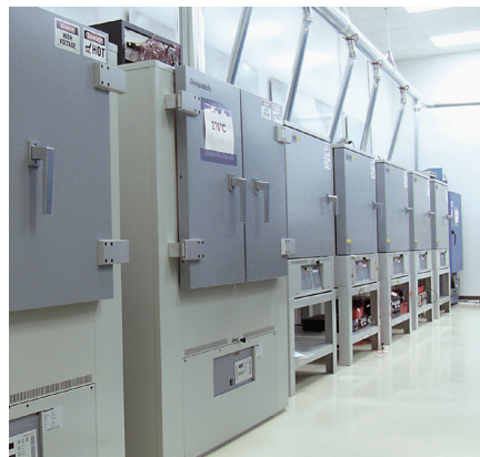
Chamber Ovens – Over 3000 cubic feet (85 cubic meters) of oven capacity is dedicated to long term thermal bias age testing. The ovens take material to temperatures above T_g . At selected intervals, samples are removed and tested to verify material integrity.
