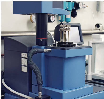
Dynamic Mechanical Analysis (DMA) – Measures the modulus of materials over a range of temperatures.
