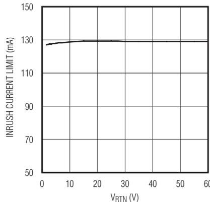
**NORMAL OPERATION CURRENT LIMIT vs.  $R_{TN}$  VOLTAGE**
