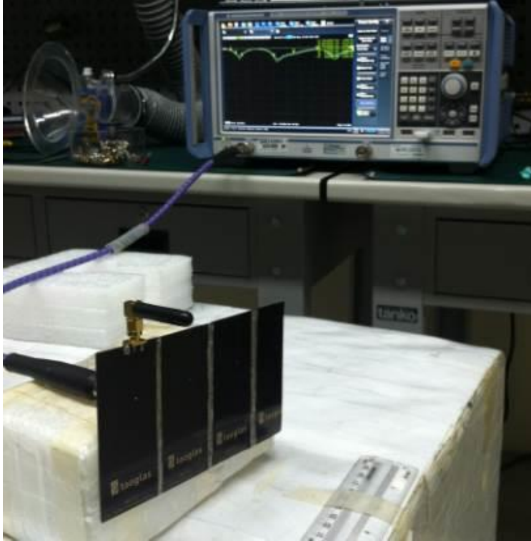
Figure 1. Impedance and VSWR measurements
