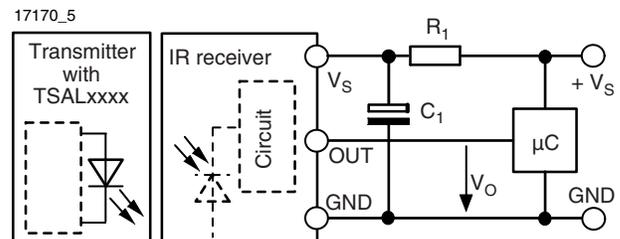
R<sub>1</sub> and C<sub>1</sub> are recommended for protection against EOS. Components should be in the range of 33 Ω < R<sub>1</sub> < 1 kΩ, C<sub>1</sub> > 0.1 µF.
