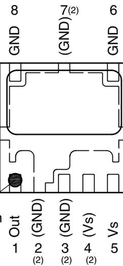
Proposed pad layout from component side (dim. for reference only)
