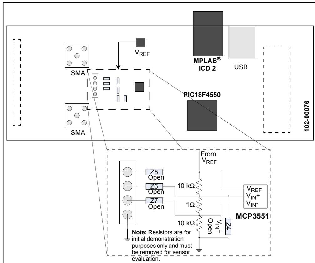
FIGURE 2-1: MCP3551 PICtail™ Demo Board Block Diagram.
