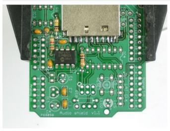
Next is the DAC (digital-analog converter) IC2. This is what turns the data into music. Make sure you pick the DAC to solder in here, it says MCP4921 on it and has a stylized M.
