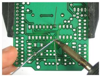
Solder the leads to the pads (metal ring) by heating both with the side-tip of the iron for 3 seconds and then poking in a bit of solder.
