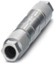
Cable connector, PROFINET CAT5 (100 Mbps), 4-pos., halogen-free, shielded, insulation displacement connection, housing material: zinc die-cast, nickel-plated, outer cable diameter of 5 mm ... 9.7 mm
