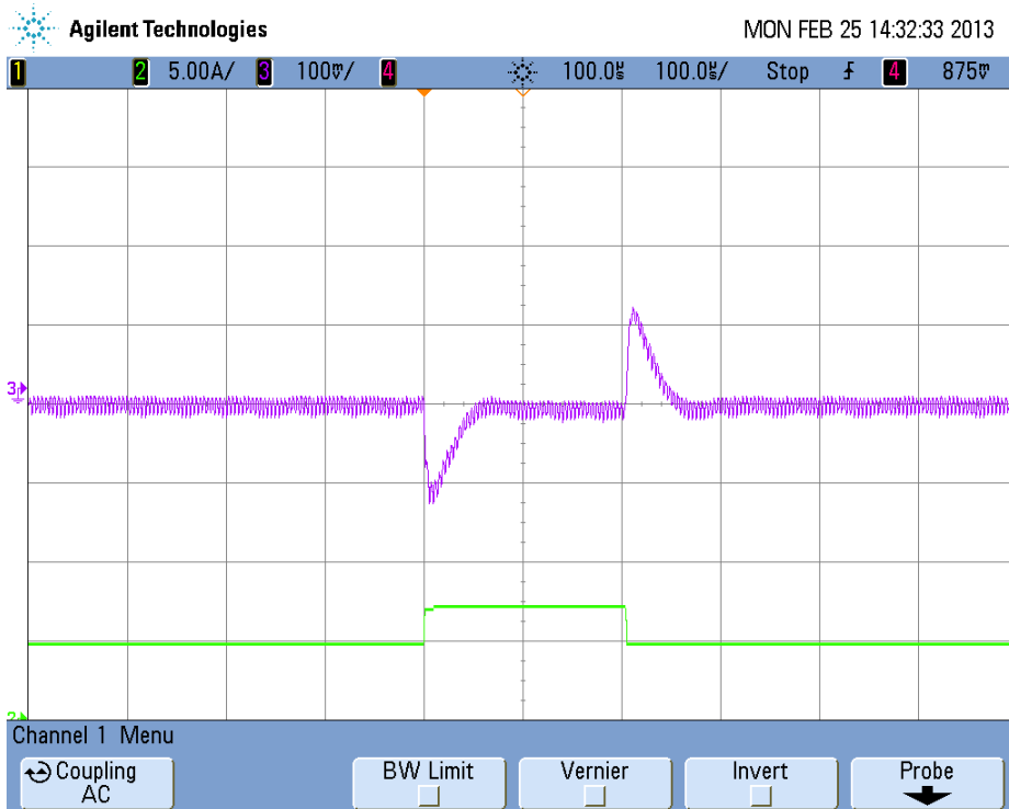
Figure 4. Transient Response Waveform at 24V IN and 5A – 7.5A – 5A OUT (5A, 100mV, 100µs/Div)
