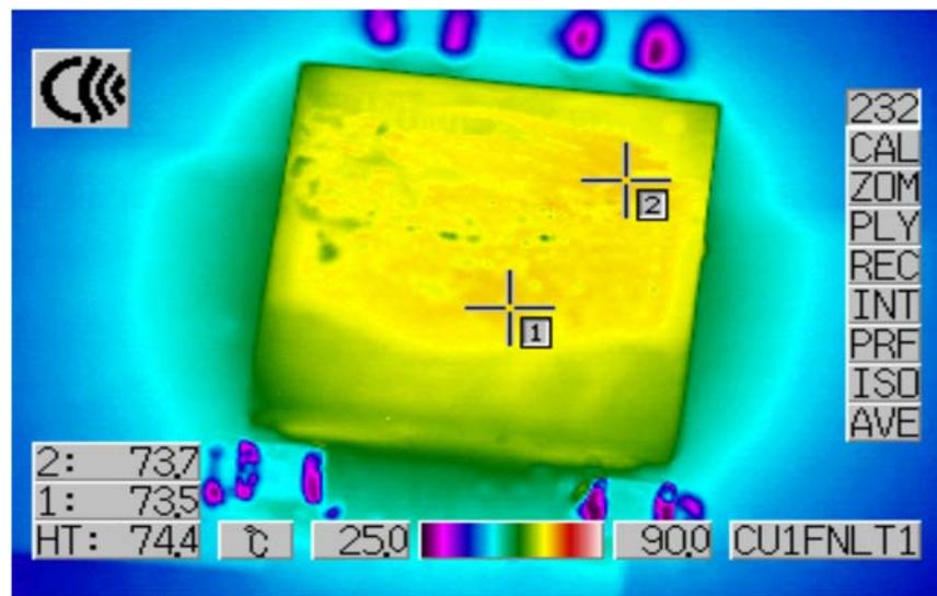
Figure 9. Thermal Capture at  $12V_{IN}$ ,  $1.5V_{OUT}$  at 12A and  $1.2V_{OUT}$  at 12A.
