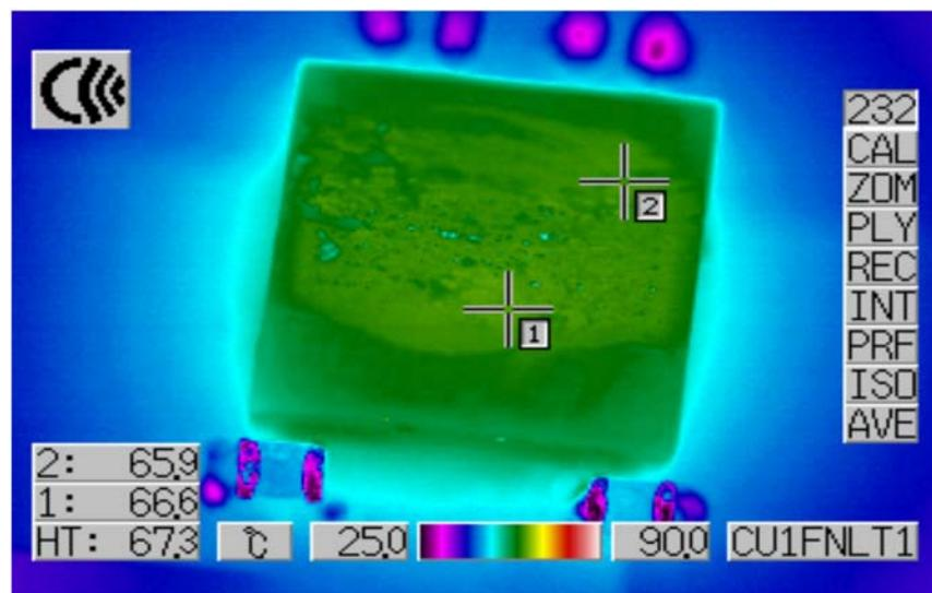
Figure 7. Thermal Capture at  $5V_{IN}$ ,  $1.5V_{OUT}$  at 12A and  $1.2V_{OUT}$  at 12A.
