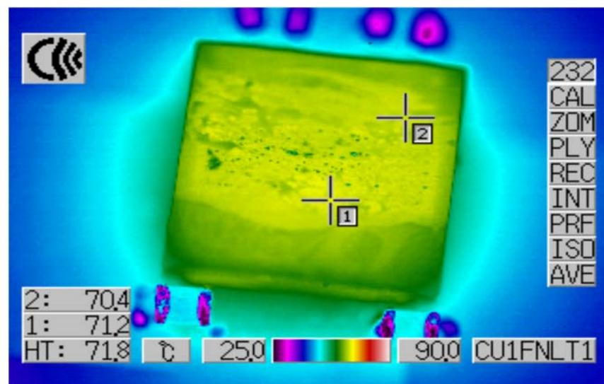
Figure 8. Thermal Capture at  $5V_{IN}$ ,  $1.5V_{OUT}$  at 13A and  $1.2V_{OUT}$  at 13A.
