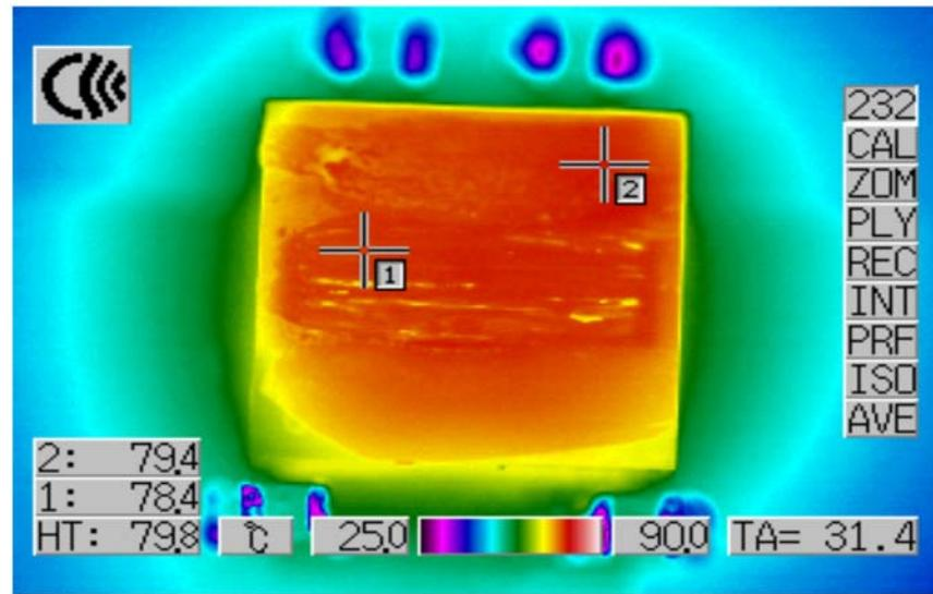
Figure 10. Thermal Capture at  $12V_{IN}$ ,  $1.5V_{OUT}$  at 13A and  $1.2V_{OUT}$  at 13A.
