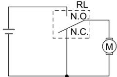
Note: NC contacts provide dynamic brake circuit
