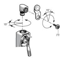
(1) Tightening torque (Min: 1) (Max: 1.5)
