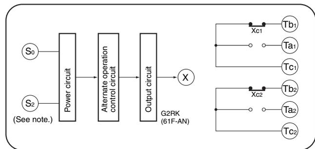
(Note: The above diagram is for a rated voltage of 200 or 220 VAC. Power is supplied to S<sub>0</sub> and S<sub>1</sub> for 100 or 110 VAC.)
