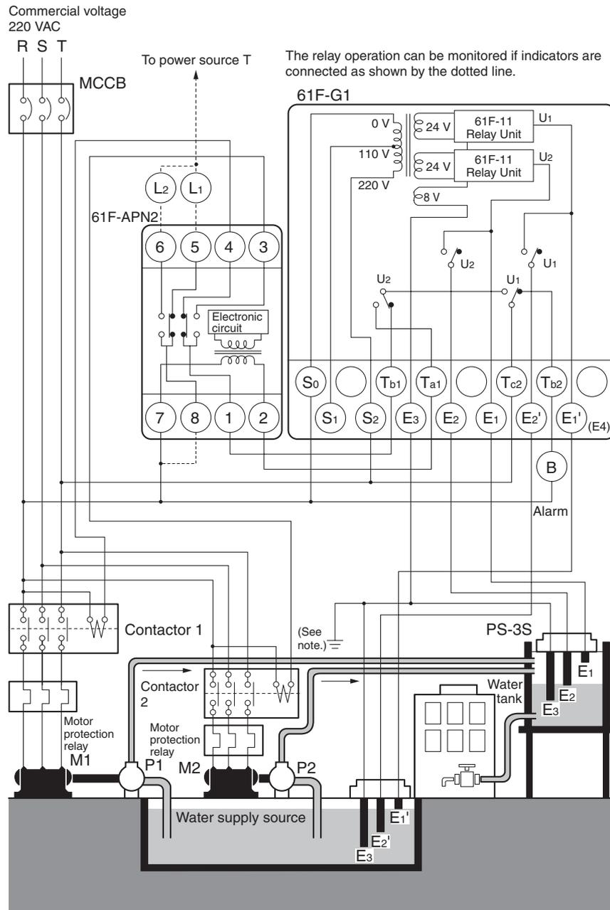
**Note:** Be sure to ground the common Electrode E<sub>3</sub> (the longest Electrode).
