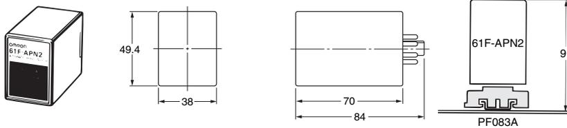
Use a PFC-N8 Mounting Bracket to mount the Level Controller to a PF083A Rail-mounted Socket.
