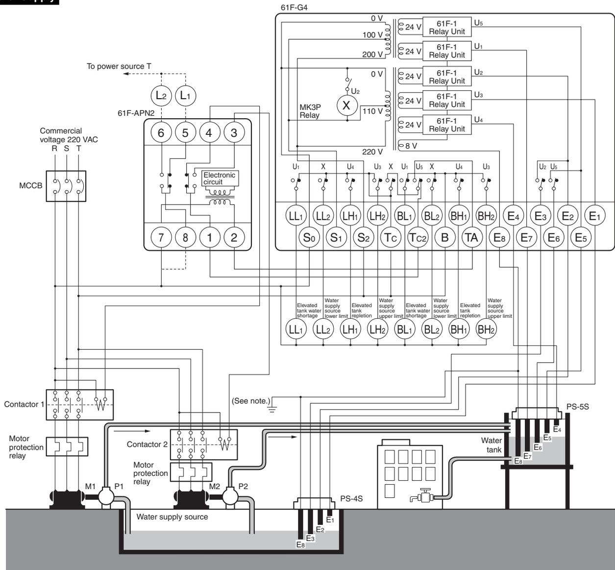
**Note:** Be sure to ground the common Electrode E<sub>3</sub> (the longest Electrode).
