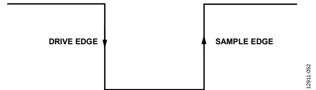
Figure 42. SPI Mode 3 SCLK Edges
