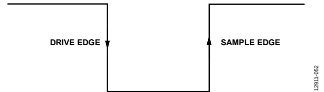
Figure 42. SPI Mode 3 SCLK Edges
