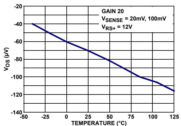
FIGURE 50.  $V_{OS}$  ( $\mu\text{V}$ ) vs TEMPERATURE
