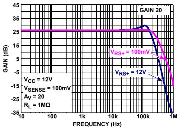
FIGURE 49. GAIN vs FREQUENCY  $V_{RS+} = 100\text{mV}/12V$ ,  $V_{SENSE} = 100\text{mV}$ ,  $V_{OUT} = 50\text{mV}_{P-P}$
