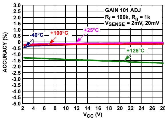
FIGURE 62. GAIN ACCURACY vs  $V_{CC}$ ,  $V_{RS+} = 12V$
