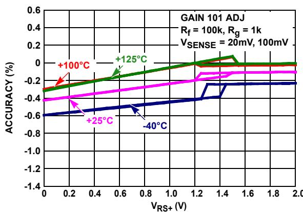
FIGURE 61. GAIN ACCURACY vs  $V_{RS+} = 0V$  TO 2V
