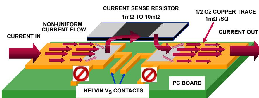
FIGURE 79. PC BOARD CURRENT SENSE KELVIN CONNECTION
