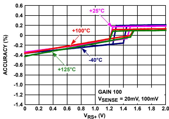
FIGURE 13. GAIN ACCURACY vs  $V_{RS+} = 0V$  TO  $2V$
