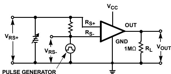
FIGURE 73.  $t_s$ , SATURATION RECOVERY TIME
