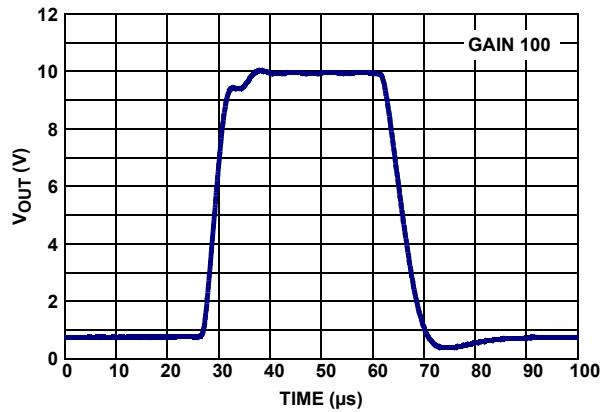
FIGURE 5. LARGE SIGNAL TRANSIENT RESPONSE  $V_{RS+} = 0.2V$ ,
