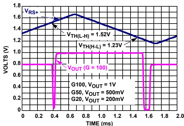
FIGURE 3. HIGH-SIDE and LOW-SIDE THRESHOLD VOLTAGE
