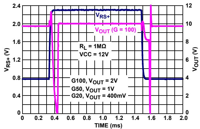
FIGURE 4.  $V_{OUT}$  vs  $V_{RS+}$ ,  $V_{SENSE} = 20mV$  TRANSIENT RESPONSE
