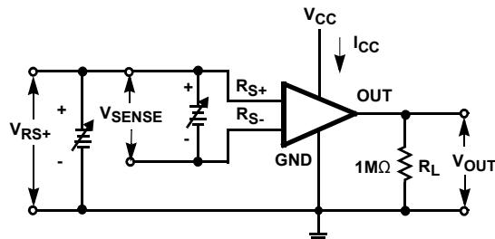
FIGURE 71.  $I_{CC}$ ,  $V_{OS}$ ,  $V_{OA}$ , CMRR, PSRR, GAIN ACCURACY
