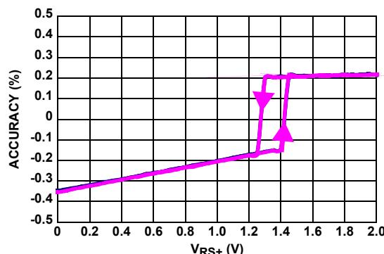
FIGURE 78. GAIN ACCURACY vs  $V_{RS+}$  = 0V TO 2V
