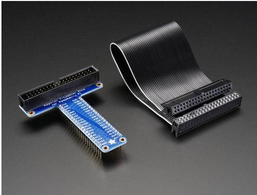
Assembled Pi T-Cobbler Plus - GPIO Breakout
