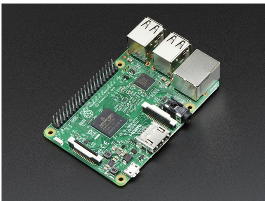
Raspberry Pi 3 - Model B - ARMv8 with 1G RAM
