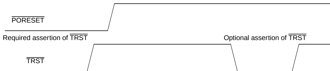
Figure 62. \overline{\text{PORESET}} vs. \overline{\text{TRST}}
