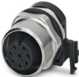
Sensor/actuator flush-type connector, socket, 8-pos., M12 SPEEDCON, A-coded, shielded, rear/screw mounting with M12 thread, with polarity protection, with angled solder connection
