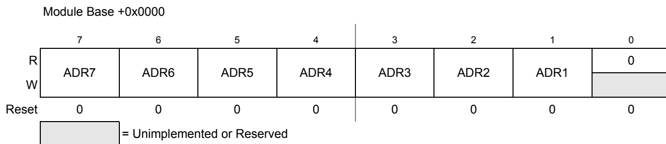
Figure 14-3. IIC Bus Address Register (IBAD)
