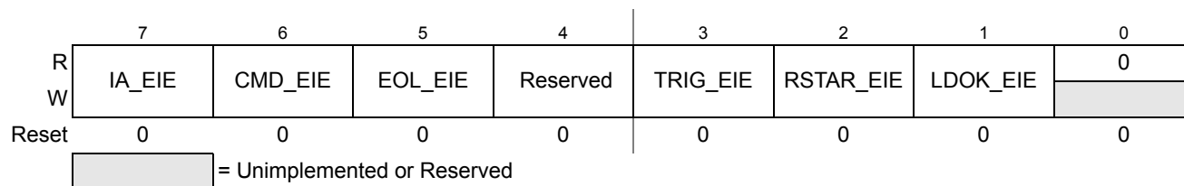
Figure 10-10. ADC Error Interrupt Enable Register (ADCEIE)
