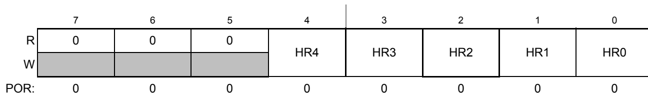
Figure 18-12. Hour Register (HRR)
