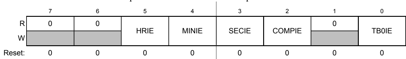
Figure 18-5. RTC Control Register 4 (RTCCTL4)
