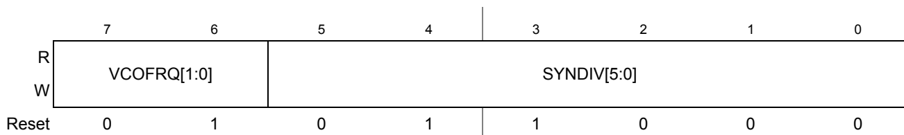
Figure 7-5. S12CPMU_UHV_V5 Synthesizer Register (CPMUSYNR)
