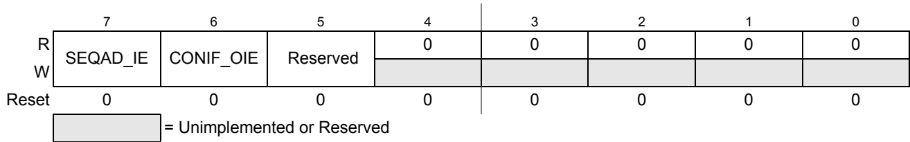
Figure 10-11. ADC Interrupt Enable Register (ADCIE)
