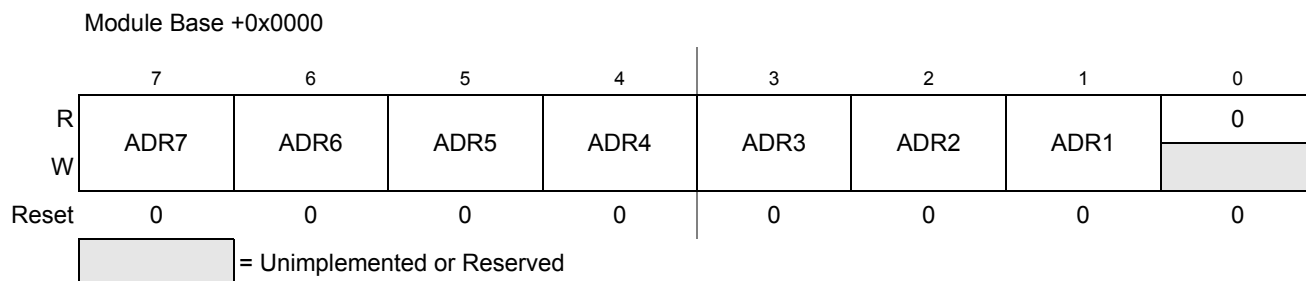
Figure 14-3. IIC Bus Address Register (IBAD)
