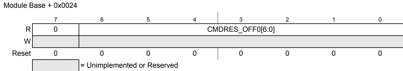
Figure 10-26. ADC Command and Result Offset Register 0 (ADCCROFF0)
