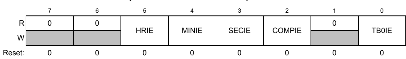
Figure 18-5. RTC Control Register 4 (RTCCTL4)
