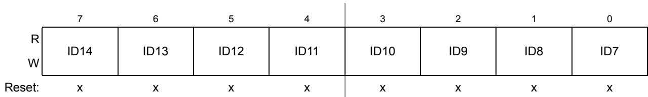
Figure 11-28. Identifier Register 2 (IDR2) — Extended Identifier Mapping
