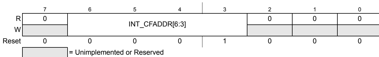
Figure 4-4. Interrupt Configuration Address Register (INT_CFADDR)
