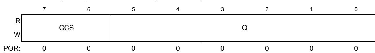
Figure 18-7. RTC Compensation Configure Register (RTCCCR)
