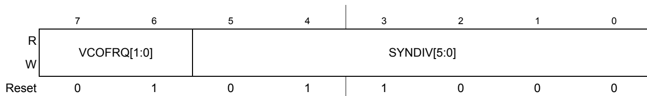
Figure 7-5. S12CPMU_UHV_V5 Synthesizer Register (CPMUSYNR)
