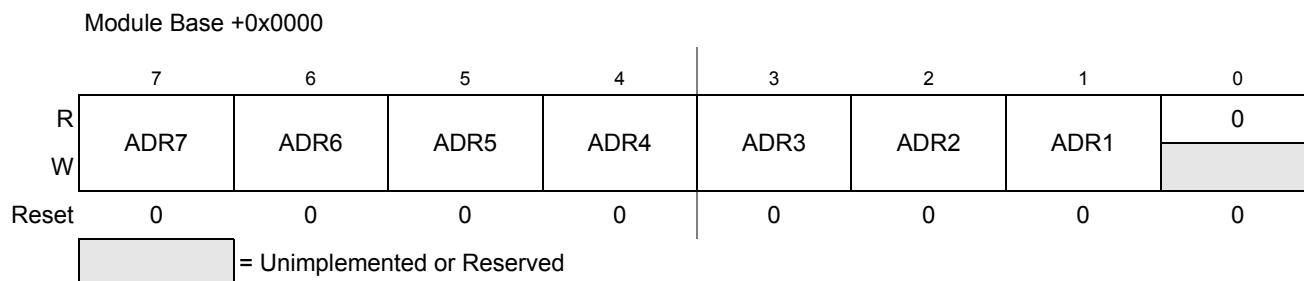
Figure 14-3. IIC Bus Address Register (IBAD)
