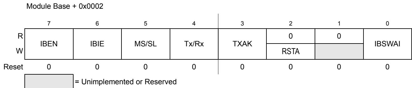
Figure 14-6. IIC Bus Control Register (IBCR)
