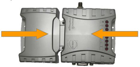
Use the 2 screws sized M2x6 and 2 spring washers, supplied together with HER040, to secure the two units in position.
