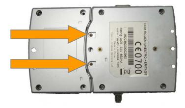
Insert SIM card, connect antenna and power supply as described in the Maestro Heritage user guide.
