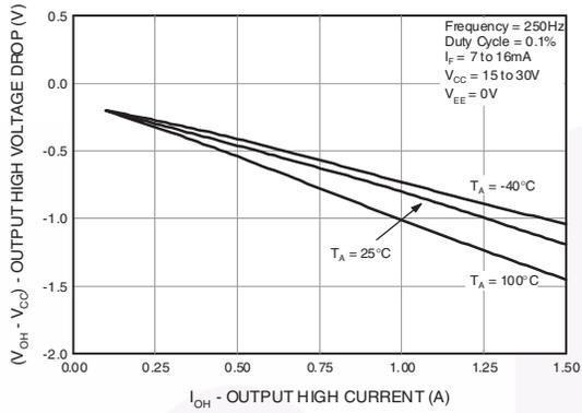
**Fig. 2 Output High Voltage Drop vs. Ambient Temperature**
