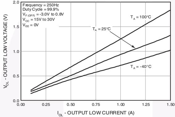
**Fig. 4 Output Low Voltage vs. Ambient Temperature**
